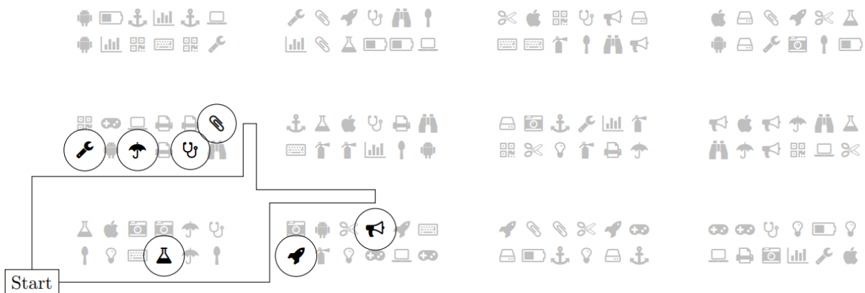
Figure 3 A warehouse layout using random stow, with SKUs stored randomly. The path shown is the shortest one that collects the 7 circled items; notice it is significantly shorter than that in the previous figure.
