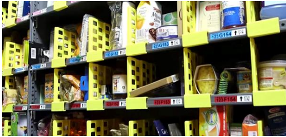
Figure 1: Random stow in a warehouse, with different items located amongst one another.
